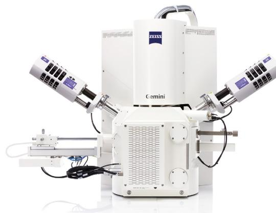
Sigma 300 is the SEM of choice for users which require enhanced resolution for particle analysis in the nanometer scale range. Sigma featuring Gemini column technology, provides outstanding imaging and analytical results from a field emission scanning electron microscope (FE-SEM). The Gemini optics provides the highest resolution imaging on a platform very well suited for elemental analysis, particularly on magnetic samples.
